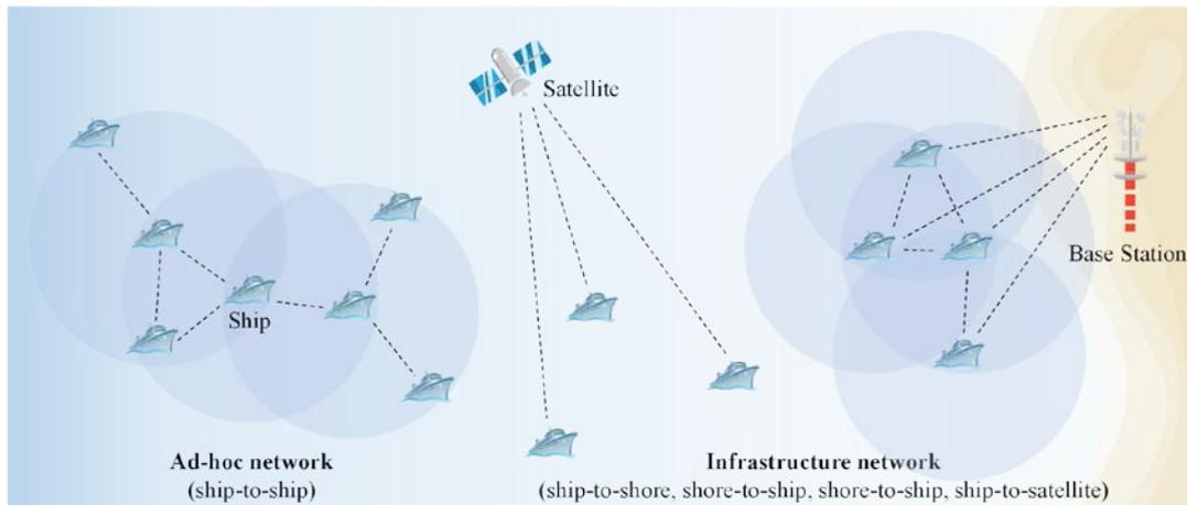
**Fig. 1.** System architecture of maritime communication network
